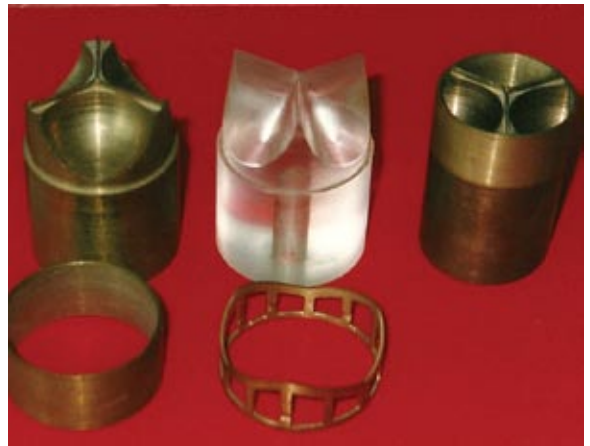
Fig 1. Moulds for building the first experimental pericardial valves
